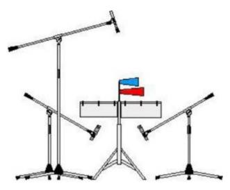
Inputs 9 and 10 placed under the timbal, pointed outwards towards the rims. Input 11 placed over the timbal on center.
